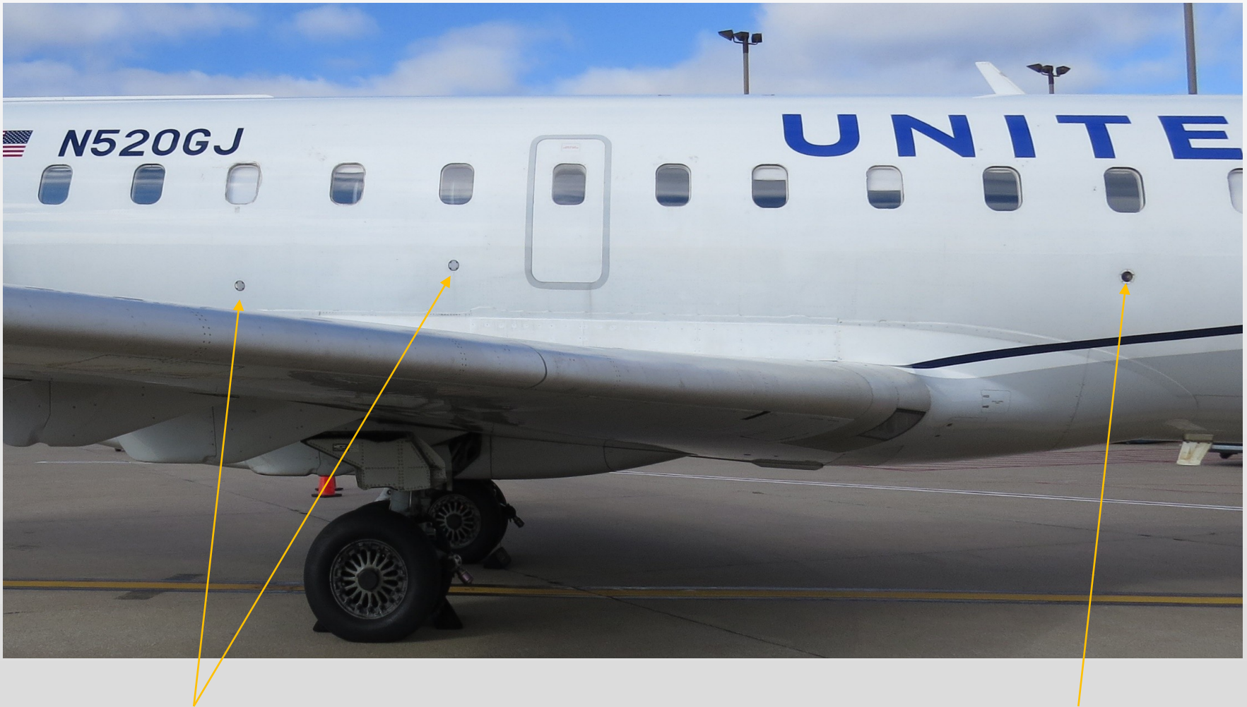
Overwing Emergency Lights
